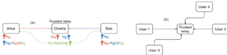
Figure 3 - Trusted relay for terrestrial QKD networks. (a) The operation principles of a trusted relay. (b) A trusted relay node offers compatibility with point-to-multipoint networks
