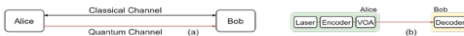
Figure 2 - Terrestrial QKD via optical fibers. (a) To avoid interference from classical channels, the quantum channel is deployed in a dedicated fiber. (b) The setup of a prepare-and-measure QKD link.
